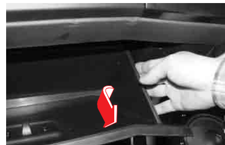
3. Push down the right side of the glove box in the direction of the arrow.
