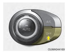
Press the front blower OFF button to turn off the front air climate control system. However, you can still operate the mode and air intake buttons as long as the ignition switch is in the ON position.
