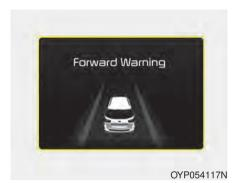
A warning message and chime will be provided when rapidly approaching a slower moving, braking or stopped vehicle ahead.
