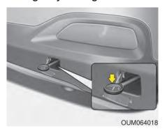
If towing is necessary, we recommend you to have it done by an authorized Kia dealer or a commercial tow truck service. If towing service is not available in an emergency, your vehicle may be temporarily towed using a cable or chain secured to the emergency towing hook under the front (or rear) of the vehicle. Use extreme caution when towing the vehicle. A driver must be in the vehicle to steer it and operate the brakes.
