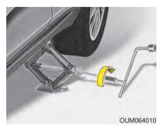
Insert the wheel lug nut wrench into the jack and turn it clockwise, raising the vehicle until the tire just clears the ground. This measurement is approximately 30 mm (1 in.).
