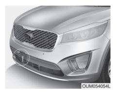
The sensor detects distance to the vehicle ahead.
