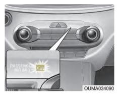
Your vehicle is equipped with an occupant detection system in the front passenger's seat.
