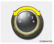
The ignition switch must be in the ON position for fan operation.
