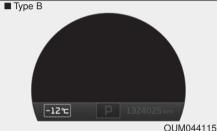
This gauge indicates the current outside air temperatures by 1°C (1°F).
