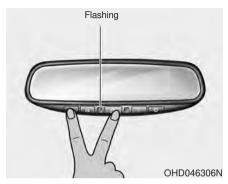
1. When programming the buttons for the first time, press and hold the left and center buttons (全, 金) simultaneously until the indicator light begins to flash after approximately 20 seconds. (This procedure erases the factory-set default codes. Do not perform this step when programming the additional HomeLink buttons.)
