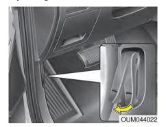
Pull the release lever to unlatch the hood. The hood should pop open slightly. Open the hood after turning off the engine on a flat surface, shifting the shift lever to the P (Park) position and setting the parking brake.
