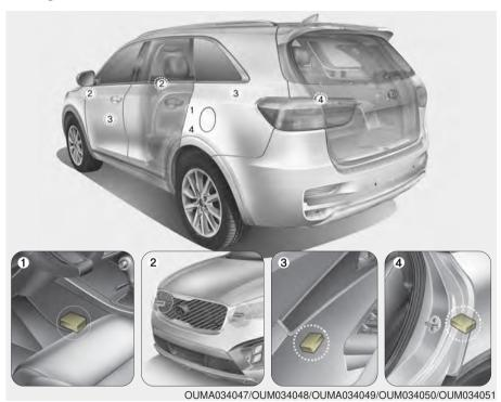
(1) SRS control module/ Rollover sensor
