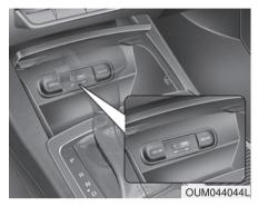
If your vehicle has an aux and/or USB(universal serial bus) port, you can use an aux port to connect audio devices, USB, or iPod®.
