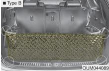
To keep items from shifting in the cargo area, you can use the holders located in the cargo area to attach the luggage net.
