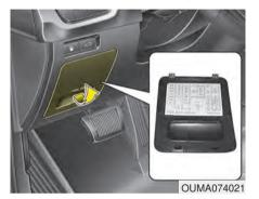
Inside the fuse/relay panel covers, you can find the fuse/relay label describing fuse/relay name and capacity.
