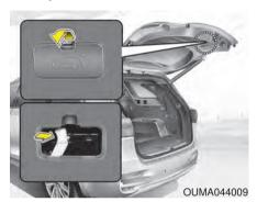
Your vehicle is equipped with an emergency liftgate (tailgate) safety release lever located on the bottom of the liftgate (tailgate). When someone is inadvertently locked in the cargo area, the liftgate (tailgate) can be opened by pushing the release lever and pushing open the liftgate (tailgate).
