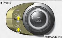
This is used to select the outside (fresh) air position or recirculated air position.
