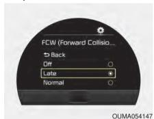
FCWS will default ON when vehicle is restarted even though FCWS was turned off on User Settings Mode.
