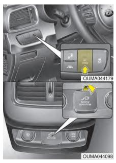
The AC inverter supplies 115V/150W electric power to operate electric accessories or equipments.
