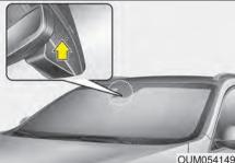
The message will appear when camera's field of view is covered by some objects. The system stops until the field of view is normal.
