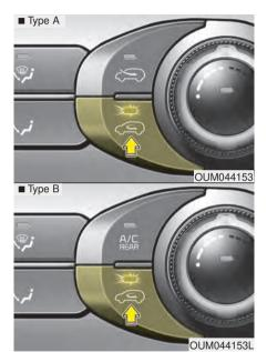
The air intake control is used to select the outside (fresh) air position or recirculated air position.
