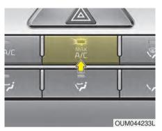
To select the MAX A/C, turn the fan speed control knob to the right then press the MAX A/C button.
