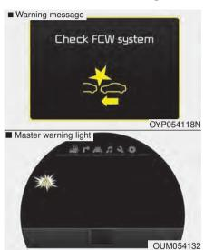
When the FCWS is not working properly, the warning message will come on for a few second. After the message disappears, the master warning light will illuminate.
