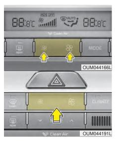
The fan speed can be set to the desired speed by operating the fan speed control button.
