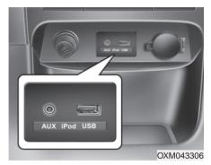
If your vehicle has an aux and/or USB(universal serial bus) port, you can use an aux port to connect audio devices and an USB and also an iPod®.
