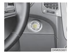
Whenever the front door is opened, the ENGINE START/STOP button will illuminate for your convenience. The light will go off after about 30 seconds when the door is closed. It will also go off immediately when the theft-alarm system is armed.
