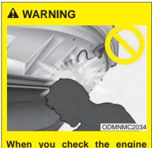
When you check the engine compartment, Take caution to avoid contacting your head with the safety hook which is located inside of the hood.
