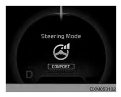
The steering wheel becomes lighter. The comfort mode is usually used when driving in the city or when parking the vehicle.
