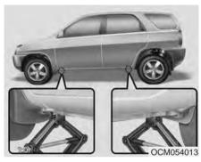
7.Place the jack at the front or rear jacking position closest to the tire you are changing. Place the jack at the designated locations under the frame.
