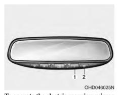
To operate the electric rearview mirror Press the I button (1) to turn the automatic- dimming function on. The mirror indicator light will illuminate. Press the O button (2) to turn the automatic- dimming function off. The
