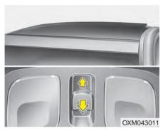
Before opening or closing the sunroof, open the roller blind (refer to the following page for instructions on how to use the roller blind).
