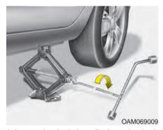
8.Insert the jack handle into the jack and turn it clockwise, raising the vehicle until the tire just clears the ground. This measurement is approximately 30 mm (1 in.).
