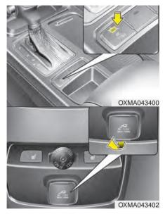
The AC inverter supplies 115V/150W electric power to operate electric accessories or equipments.
