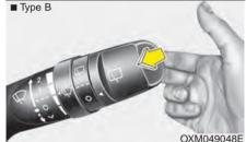
In the OFF position, pull the lever gently toward you to spray washer fluid on the windshield and to run the wipers 1-3 cycles.
