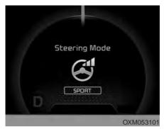
The steering wheel becomes heavier. The sport mode is usually used when driving on the highway.
