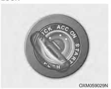
The steering wheel locks to protect against theft (if equipped). The ignition key can be removed only in the LOCK position.
