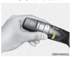
Fog lights are used to provide improved visibility when visibility is poor due to fog, rain or snow, etc. The fog lights will turn on when the fog light switch (1) is turned to the on position after the headlight is turned on.
