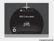
The message will appear to notify the driver if there are foreign substances on the rear bumper or it is hot near the rear bumper. The light on the switch and the system will turn off automatically.
