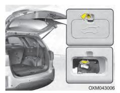
Your vehicle is equipped with an emergency tailgate safety release lever located on the bottom of the tailgate. When someone is inadvertently locked in the cargo area, the tailgate can be opened by pushing the release lever and pushing open the tailgate.
