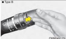
Push the lever away from you to spray rear washer fluid and to run the rear wipers 1~3 cycles. The spray and wiper operation will continue until you release the lever
