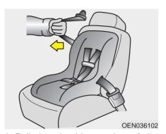
Pull the shoulder portion of the seat belt all the way out. When the shoulder portion of the seat belt is fully extended, it will shift the retractor to the "Auto Lock" (child restraint) mode.
