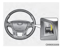
If any method other than the CRUISE button was used to cancel cruising speed and the system is still activated, the most recent set speed will automatically resume when you move the lever up (to RES+).
