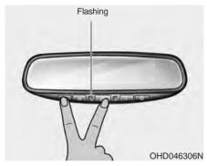
1. When programming the buttons for the first time, press and hold the left and center buttons (① ① ① 10) simultaneously until the indicator light begins to flash after approximately 20 seconds. (This procedure erases the factory-set default codes. Do not perform this step when programming the additional HomeLink buttons.)
