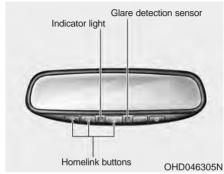
HomeLink® Wireless Control System Your new mirror comes with an inte-HomeLink arated Universal Transceiver, which allows you to program the mirror to activate your garage door(s), estate gate, home lighting, etc. The mirror actually learns the codes from your various existing transmitters.
