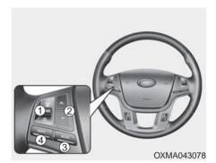
The steering wheel may incorporate audio control buttons. These buttons are installed to promote safe driving.
