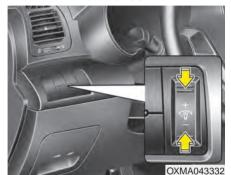
The brightness of the instrument panel illumination is changed by pressing the illumination control button ("+" or "-") when the ignition switch or Engine Start/Stop button is ON, or the tale lights are turned on.
