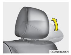
6. Also, unfold the headrest manually.
