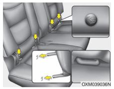
LATCH anchors have been provided in vour vehicle. The LATCH anchors are located in the left and right outboard rear seating positions. Their locations are shown in the illustration. There is no LATCH anchor provided for the center rear seating position.
