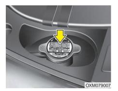
**WARNING** - Radiator cap Do not remove the radiator cap when the engine and radiator are hot. Scalding hot coolant and steam may blow out under pressure causing serious injury.
