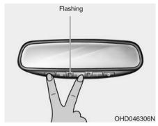
1. When programming the buttons for the first time, press and hold the left and center buttons ( ①, ①) simultaneously until the indicator light begins to flash after approximately 20 seconds. (This procedure erases the factory-set default codes. Do not perform this step when programming the additional HomeLink buttons.)
