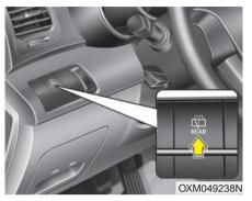
Press the button to spray rear washer fluid and to run the rear wipers.
