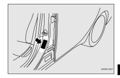
This placard shows the maximum number of occupants permitted to ride in your vehicle as well as "the combined weight of occupants and cargo" (A), which is called the vehicle capacity weight. The weight of roof road is included in the definition of "cargo" when determining the vehicle capacity weight. This placard also tells you the size and recommended inflation pressure for the original equipment tires on your vehicle. For more information, refer to "Tires" on page 9-17.
