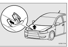
Release the safety lever and lift the engine
