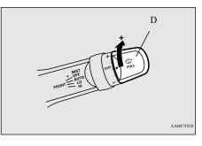
The wipers will operate once if the lever is moved to the "AUTO" position and the knob
