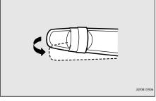
4. The headlights will come on in the low beam setting for about 30 seconds. After the headlights go off, the headlights can be turned on again in the low beam setting for about 30 seconds by pulling the turn signal lever toward you within 60 seconds of turning the ignition switch to the "LOCK" position. To turn on the headlights again after 60 seconds of turning the ignition switch to the "LOCK" position, repeat the process from step 1.
