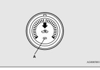
When the air conditioning turns on, the air selection is controlled automatically. The air selection indicator light (A) shows the selected position.
