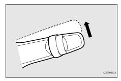
The wipers will operate once if the wiper lever is raised to the "MIST" position and released. This operation is useful when it is drizzling, etc. The wipers will continue to operate while the lever is held in the "MIST" position.
