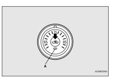
When the air conditioning turns on, the air selection is controlled automatically. When the air conditioning turns off, the air selection automatically goes back to the outside air position.
