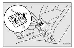
1- Heater high (for quick heating)
