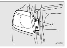
2. Remove the light unit in the rear direction.
