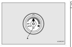
Push the switch again and the air conditioning compressor will stop and the indicator light (A) goes off.
