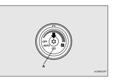
Push the switch again and the air conditioning compressor will stop and the indicator light (A) goes off.
