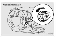
For vehicles with a continuously variable transmission (CVT) or Twin Clutch SST, when removing the key, first set the selector lever (CVT) or the gearshift lever (Twin Clutch SST) to the "P" (PARK) position, and then turn the key to the "LOCK" position and remove it.
