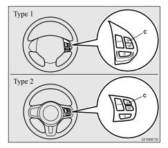
To increase the speed in small amounts, press the "ACC RES" switch (C) for less than 1 second and release it. Every time you press the "ACC RES" switch (C), the speed will increase by approximately 1 mph (1.6 km/h).
