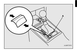
When the engine is started, the control mode is automatically set to the "Normal" mode. Use the following procedures to change the control mode.
