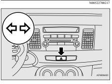
If you press the flasher switch, the front and rear turn signals will flash intermittently, and so will the hazard warning lights. This is an emergency warning system and should not be used when the vehicle is in motion, except for emergencies.
