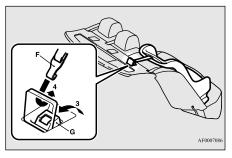
5. Push and pull the child restraint system in all directions to be sure it is firmly secured.
