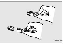
4. Use the fuse location diagrams and the matching tables, to check the fuse that is related to the problem. If the fuse is not blown, something else must be causing the problem. Contact an authorized Mitsubishi Motors dealer or a repair facility of your choice to have the problem checked.
