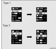
3. Press and hold the multi-information meter switch (for about 2 seconds or more) to switch in sequence from ON (operation sound on)  $\rightarrow$  OFF (operation sound off)  $\rightarrow$  ON (operation sound on). The setting is changed to the selected condition.
