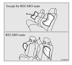
A label is attached to the seatbacks in vehicles with side airbags.
