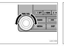
Turn the PWR/VOL key clockwise to increase, and counter- clockwise to decrease the volume.
