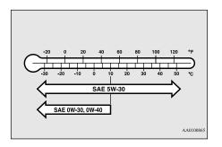
Mitsubishi Motors Genuine 5W-30 Engine Oil is the recommended oil for optimum engine performance and protection. SAE 0W-30 or 0W-40 engine oil is recommended to improve engine starting in cold weather conditions. Refer to temperature chart.
