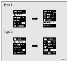
3. Press and hold the multi-information meter switch for about 2 seconds or more to switch in sequence from 1 (turn signal sound 1)  $\rightarrow$  2 (turn signal sound 2)  $\rightarrow$  1 (turn signal sound 1).
