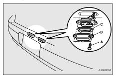
2. Remove the socket and bulb assembly together by turning it counterclockwise.
