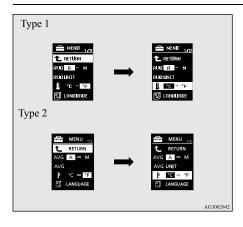
3. Press and hold the multi-information meter switch (for about 2 seconds or more) to change in sequence from  $^{\circ}F \rightarrow ^{\circ}C \rightarrow ^{\circ}F$ .
