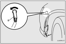
4. Pull the bulb out of the socket.
