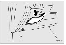
2. For vehicles with the bottom cover, use the puller to loosen the 2 clips (A) and push down the bottom cover. The puller is in the fuse block in the engine compartment. Refer to "Fuse replacement" on page 9-33.
