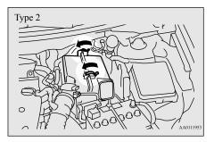
5. Install the air cleaner filter and put the cover back on in its original position.
