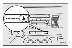
When the key is turned to the "ON" position, this indicator normally comes on and goes off a few seconds later.
