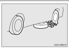
2. To remove the spare tire, remove the installation clamp (C) by turning it counterclockwise.
