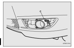
3. Push the connector (D) to disconnect and remove the fog light.
