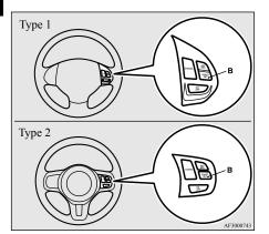
To decrease the speed in small amounts, press the "COAST SET" switch (B) for less than 1 second and release it. Every time you press the "COAST SET" switch (B), the speed will decrease by approximately 1 mph (1.6 km/h).
