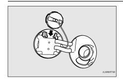
7. To close, turn the fuel tank filler cap slowly clockwise until you hear clicking sounds, then gently push the fuel tank filler door closed.
