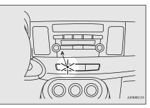
4. The system has entered the armed stage after about 20 seconds, when the theftalarm indicator (A) flashing becomes slower.
