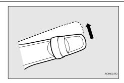
The wipers will operate once if the lever is raised to the "MIST" position and released when the ignition switch is in the "ON" or "ACC" position. The wipers will continue to operate while the lever is held in the "MIST" position.
