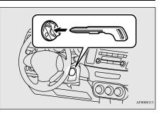
4. Insert the F.A.S.T.-key into the emergency key.
