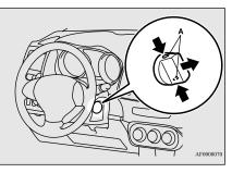
3. Insert the emergency key into the ignition switch.
