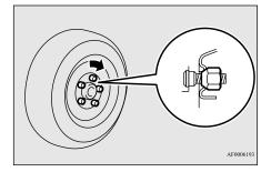
[Vehicle with aluminum wheels] • Normal wheels Temporarily tighten the wheel nuts (flange nuts) until their flange section comes in contact with the wheel and it is no longer loose.
