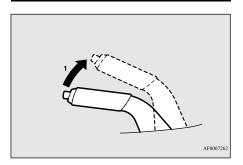
Pull the lever up without pushing the button at the end of hand grip.
