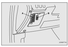
A- Main fuse blockB- Sub fuse block
