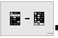
3. Press and hold the multi-information meter switch for about 2 seconds or more to switch in sequence from ON (with the green bar graph)  $\rightarrow$  OFF (without the green bar graph)  $\rightarrow$  ON (with the green bar graph).
