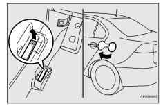
3. Open the fuel tank filler pipe by slowly turning the cap counterclockwise.
