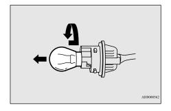
5. To install a bulb, perform the removal steps in reverse.
