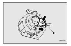
5. Remove the bulb assembly (E) by turning it counterclockwise.
